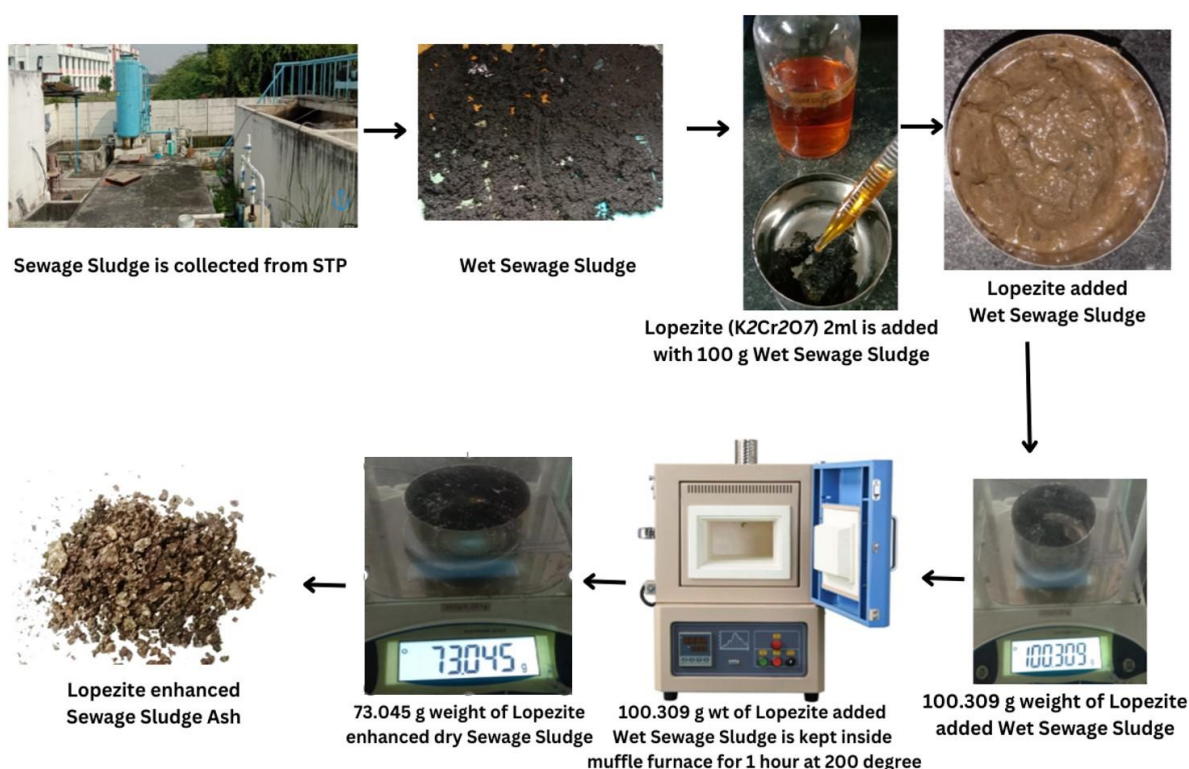
Figure 1. The Process of Making Lopezite enhanced Sewage sludge ash
