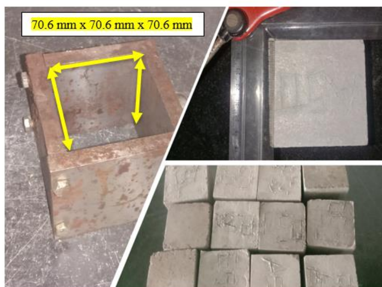
Figure 7. 70.6 mm x 70.6 mm x 70.6 mm cube mould and casted specimens
