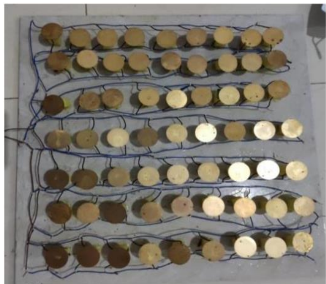
Figure 10. Parallel circuit of piezoelectric transducer
