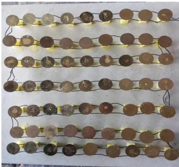
Figure 9. Series circuit of piezoelectric transducer
