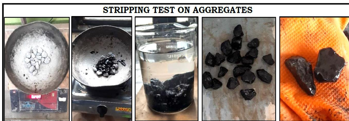
Figure 3. Stripping test on aggregates
