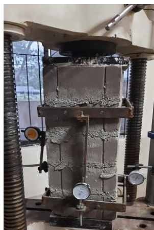
Figure 6. Experimental setup for testing of solid block masonry prism
