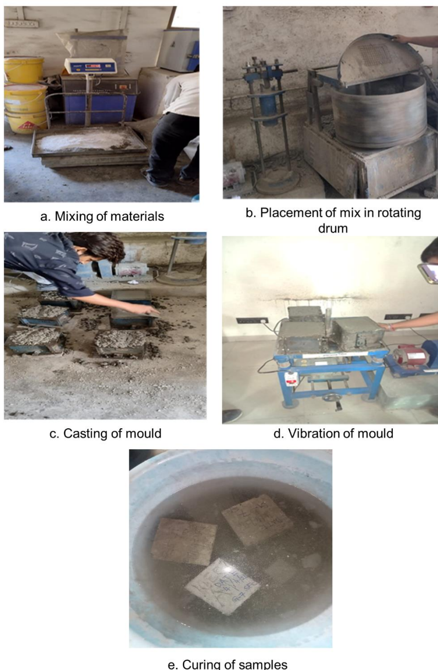
Figure 4. Various stages involved in study from of mix preparation to curing
